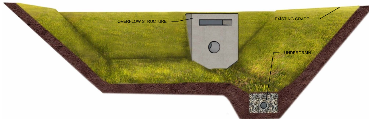
Figure 4.4 Floodplain Detention System Concept
