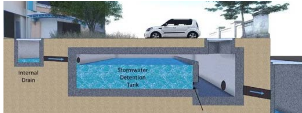
Figure 4.5 Detention Basin Facility Concept. Stormwater Sydney
